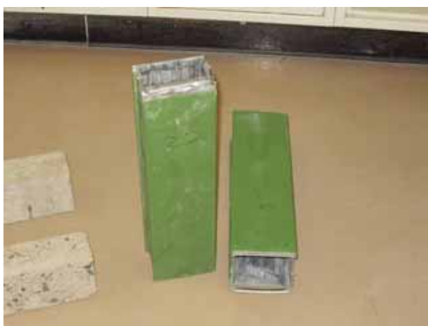
Figure 8. Photo. Vertical container for freeze-thaw concrete specimen (ASTM C 666 Procedure A).
