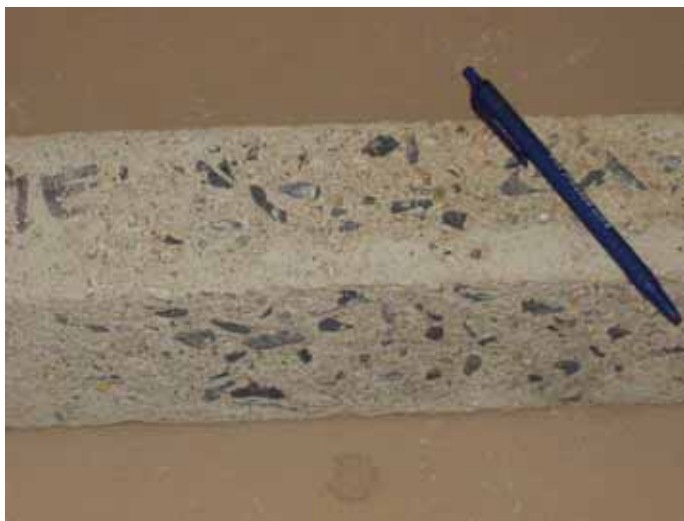
Figure 37. Photo. Scaling of typical specimen. The specimens tended to scale toward the center region of the beam specimens corresponding to the area where the metal containers bulged due to ice formation between the concrete and the container.
